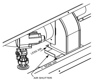
Figure 52 – Adjusting Air Shutter 500,000 - 750,000 Btu/hr
